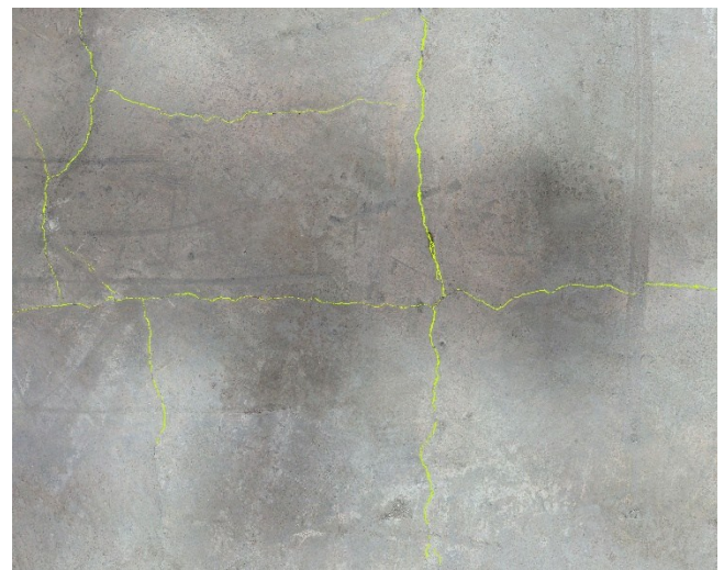
Figure 2. The finalized crack map – the composition of crack pixels onto the texture space
