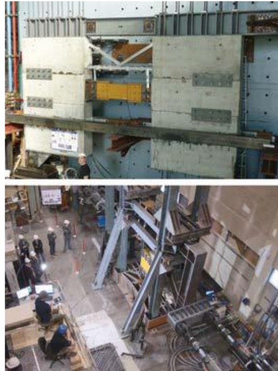
Figure 7. Full-Scale VCD Tests at the University of Toronto
