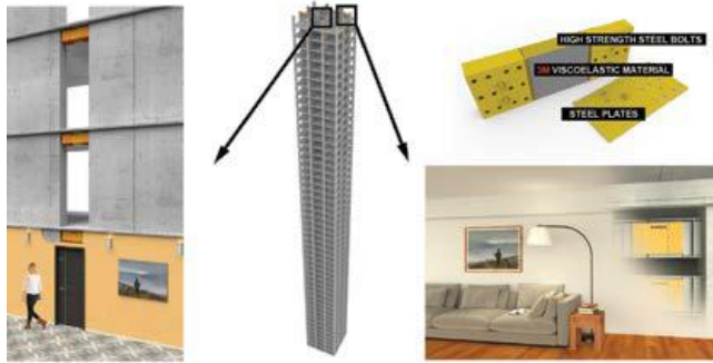
Figure 5. VCD Schematics in core wall and outrigger configurations
